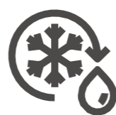
Automatic defrosting ensures the evaporator working to its optimum performance. Automatically vaporizing the defrosted water
